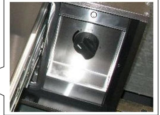
The temperature range of the warming drawer is between **90° F (Min) to 250° F (Max)**. The temperature is control by the thermostat. In order to gain access to the thermostat and power connections, removed the unit from the cabinet to expose the right side access panel. **FIG 3** shows the cover installed (Outlined with dotted red line)
